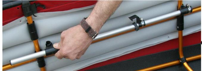
**4.** Install the rail on the other side of the canoe to match the placement of the rail you just installed.
