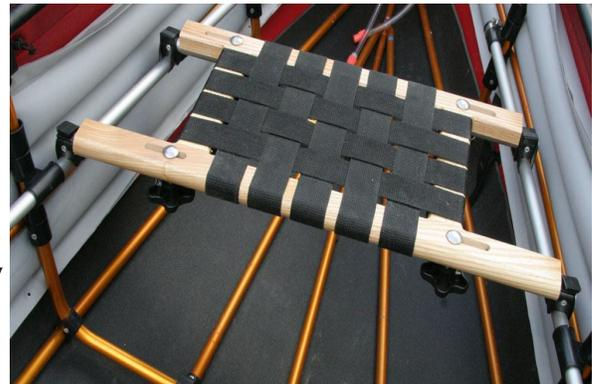
**7.** A revised style of the PakCanoe seat offers a wider range of adjustment. The seat's adjustment is fixed with a screw driver by tightening stainless clamps that compress the tubular sleeves under the seat to prevent any side to side movement. The clamps are secured to the seat frame. No adjustments need to be disturbed when the canoe is disassembled, and no tool is needed to reassemble the canoe.
